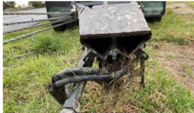
Figure 2. Broken draw bar – critical risk
