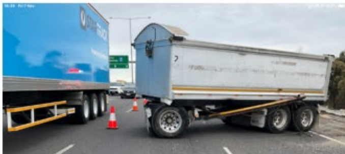
Figure 1. Broken draw bar – critical risk
